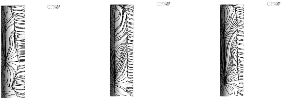
Figure 5: Surface streamlines at a left oblique view of the cylinder - From left to right - URANS, DES and LES
